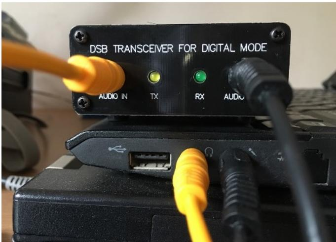
**FOR LEGACY COMPUTERS WITH SEPARATED MIC AND HEADPHONE CONNECTORS, JUST CONNECT AUDIO IN TO HEADPHONE CONNECTOR, AND AUDIO OUT TO MIC CONNECTOR.**
