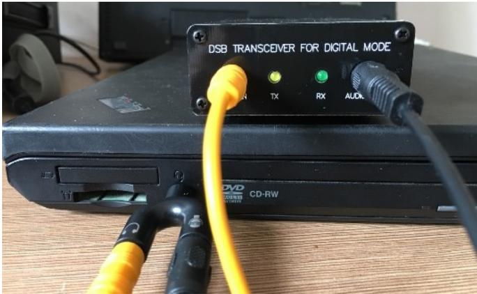
**FOR MODERN COMPUTERS WITH SINGLE CONNECTOR FOR HEADSET, USE Y-ADAPTER TO MAKE CONNECTION. Y-ADAPTER IS AVAILABLE**
