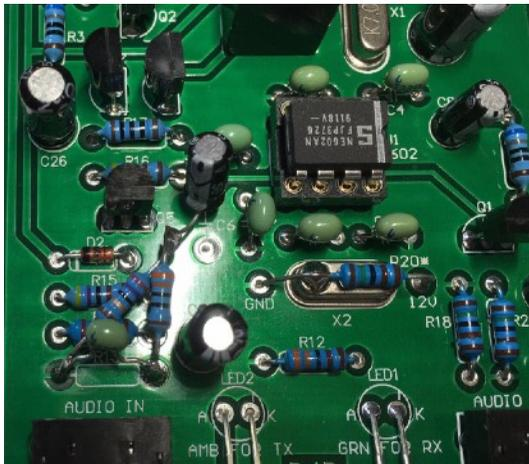
2. Improve carrier leakage by cutting a trace near 78L05 and adding a 1N4148 diode to reduce power supply voltage of NE602 by about 0.7V. This is the idea from BH4DCL and my test shows very effective result without noticeable side effects.
